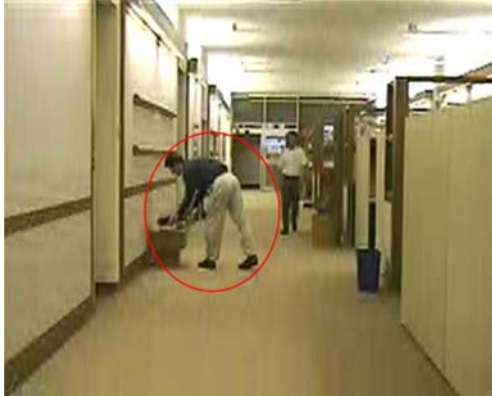
Figure 18 Perceptual quality given by MPEG 4 coding at 130 Kbps (Hall Monitor, 114th frame) (see online version for colours)
